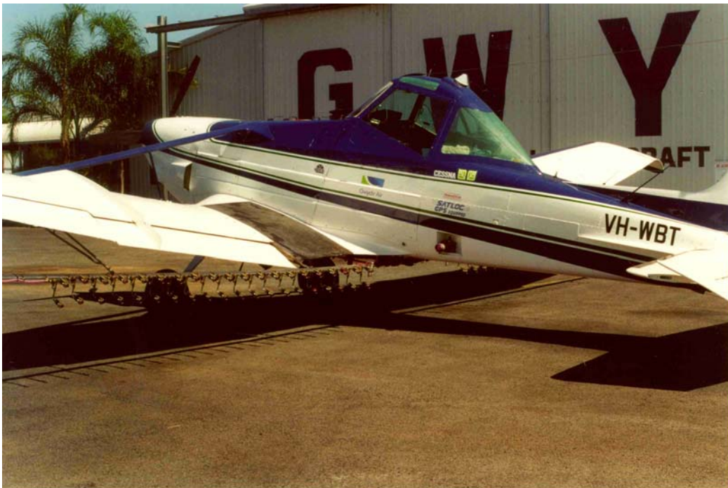
The aircraft fitted with the 80 spectrum electrostatic nozzles prior to the trial
