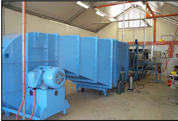
Wind tunnel (fan, settling chamber and working section)
